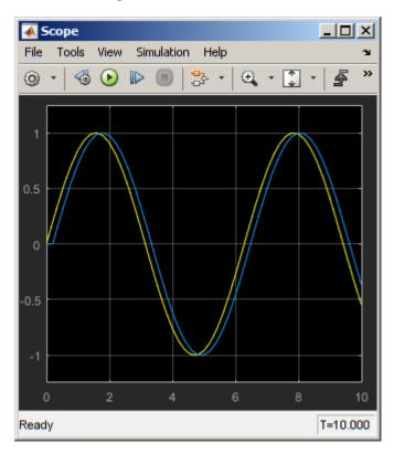
The Scope shows that the Sine Wave signal is delayed by only one sample. The OPC Write block's priority is set higher than the OPC Read block to ensure that the read operation occurs after the write operation. This ensures only one sample delay between the write and read operation.
