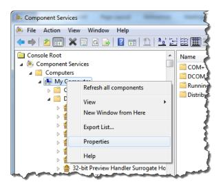
In the **Default Properties** tab, make sure that Enable Distributed COM On This Computer is selected. Select None as the Default Authentication Level, and Anonymous as the Default Impersonation Level.
