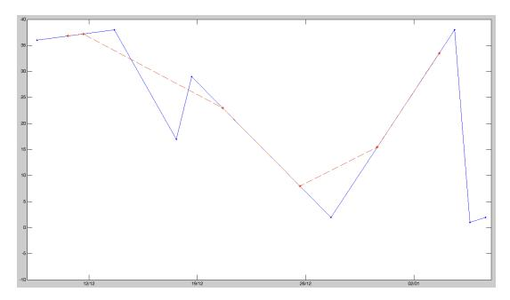
In this figure, the blue line represents the original data values while the red line represents the resampled data at a new set of timestamps. These new timestamps are marked by red stars while the original timestamps are marked by blue circles.
